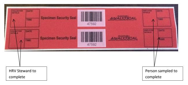
4.19 The HRV Steward, who collected the sample, should seal both specimens immediately by placing a specimen security seal over the lid of each bottle (barcoded number over cap), with the ends pressed firmly down on either side of the bottle. (See below image)
